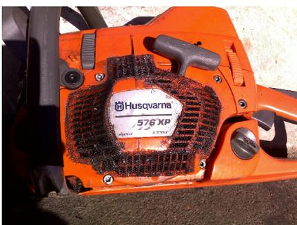
**Tip # 4: Keep the plastic chips out of the engine cooling system.**
