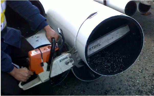
Not so long ago it was discovered that chainsaws are one of the best, most efficient tools for cutting medium to large diameter poly pipe as used extensively in the mining and irrigation industries.
